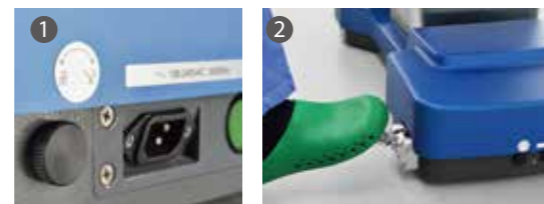
Step 1: Turn the knob clockwise to enter the Manual Override System mode.
